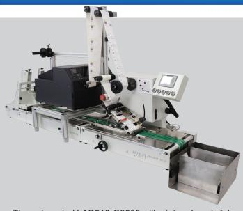
The automated LAB510-C6500 will print and apply fully coloured labels to a wide variety of products up to 3000 pieces per hour! The LAB510 can label any type of box, envelopes, cartons, phone or scratch off cards, lottery tickets, vouchers, in fact any product with a flat surface and a maximum height of 2,36" (60mm) and width of 12.4" (310mm).
